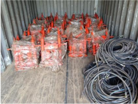
Turret 12MT Tank Bygging Jacks & Connecting Hoses
